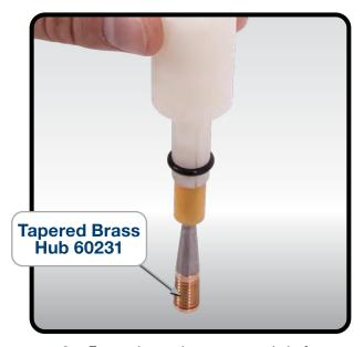
3. Force sleeve down onto tool shaft
