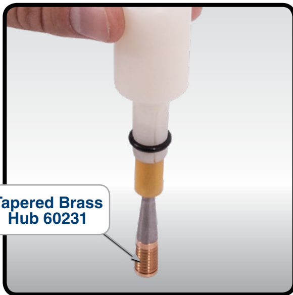
3. Force sleeve down onto tool shaft
